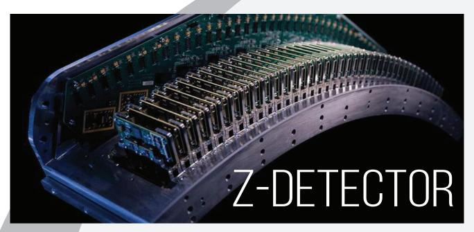
The Z-Detector, designed with a fully integrated architecture and powered by through-silicon via (TSV) technology, shortens the signal transmission path from cm-level to µm-level. The outstanding denoising performance substantially improves the signal-to-noise ratio (SNR) and significantly enhances the capability to capture fine details within images.
