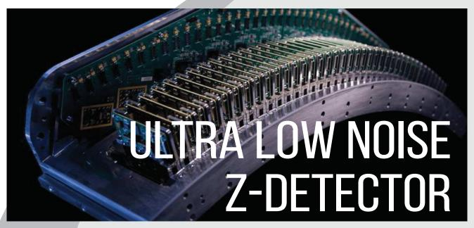
The Z-Detector greatly shortens the signal transmission path and produces a highly-stable digital signal, based on its advanced design. The Z-Detector reduces image noise and delivers excellent image quality along with a low radiation dose. The 22 mm of coverage of the Z-Detector, coupled with a 0.5 second rotation speed, enables the uCT 530 to complete the scan in a
