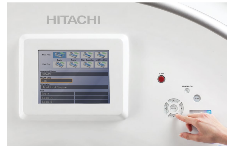
Review and update patient information at the gantry and start and pause scans
